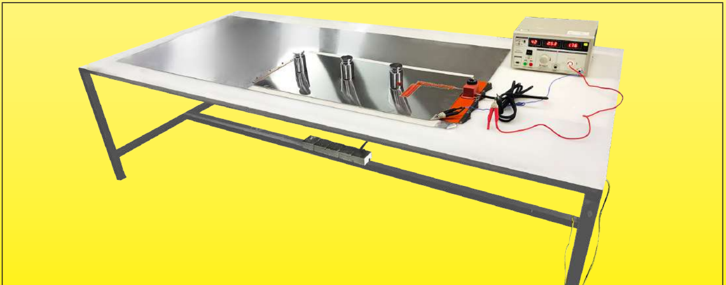
Measuring equipment for total current leakage at cold condition
